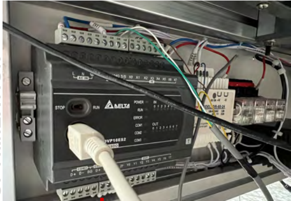
Delta dvps2 series. The WPLSoft software is used to compile the program, which is then input into the single-chip microcomputer.
