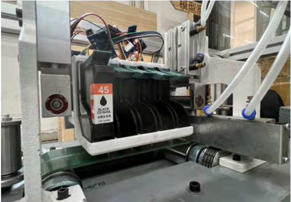
The printing device consists of 5 ink cartridges, 5 ink cartridge controller, and a protective case made by 3d printing.
